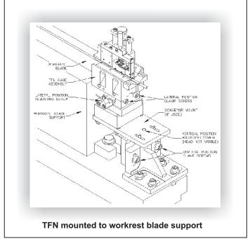
The TFN can also be mounted to a conveyor attached to the workrest blade. This eliminates problems with backpressure on the parts flowing out from between the grinding wheels. If the machine is designed so the workrest blade moves during compensation, a linear bearing supports the conveyor and allows it to move laterally with the machine slide.
