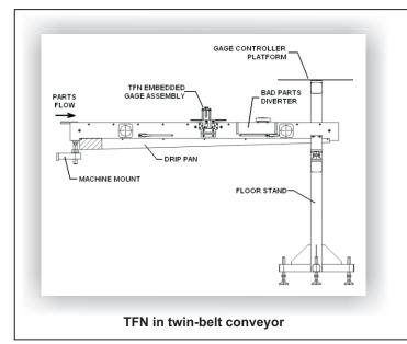
For on-machine mounting, the TFN is supported by a bracket mounted to the workrest blade support. The bracket includes horizontal and vertical adjustments for alignment to the work blade. It may also include attachments for mounting a transfer conveyor for moving the parts away from the grinder or further on in the production line.
