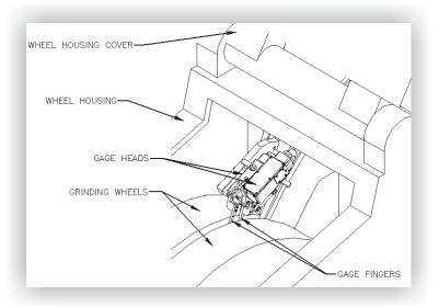
On horizontal spindle machines, gages are accessed from the top. These gages are built rugged to live in this environment.
