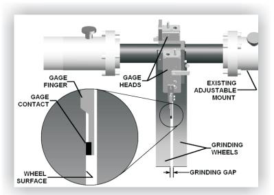
Dual wheel gage on this disc grinder controls grind-line (both wheels) plus part size (by maintaining the correct grinding gap)
