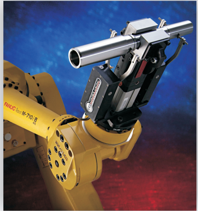
Robot gripper with two gage heads measures diameters while part is moved to next operation
