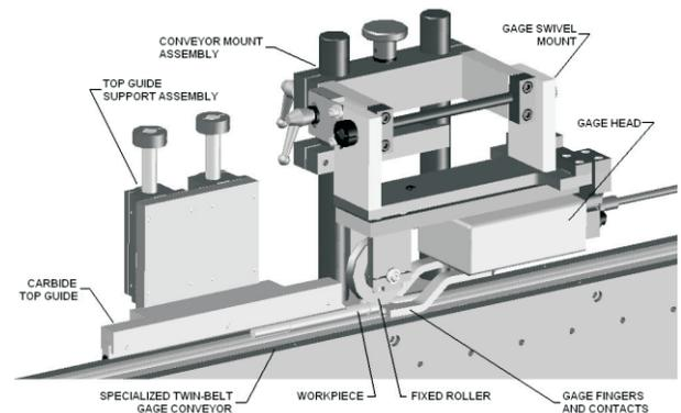
**TFD-24 with auxiliary carbide top for a mix of long and short parts**
